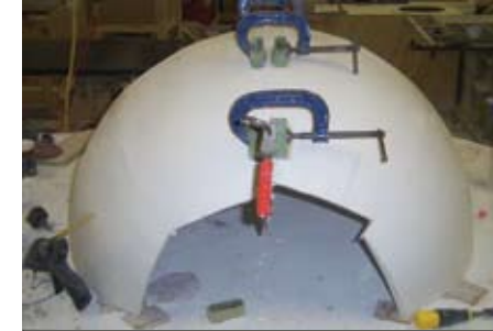
Assembly of 2 quarter pieces to half a shell
