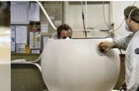
Final sanding of the shell
