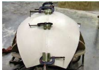
Seaming of 2 segments to make a quarter
