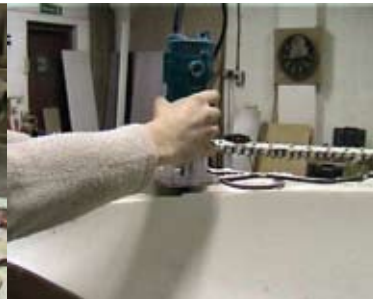
Seam preparation by trimming
