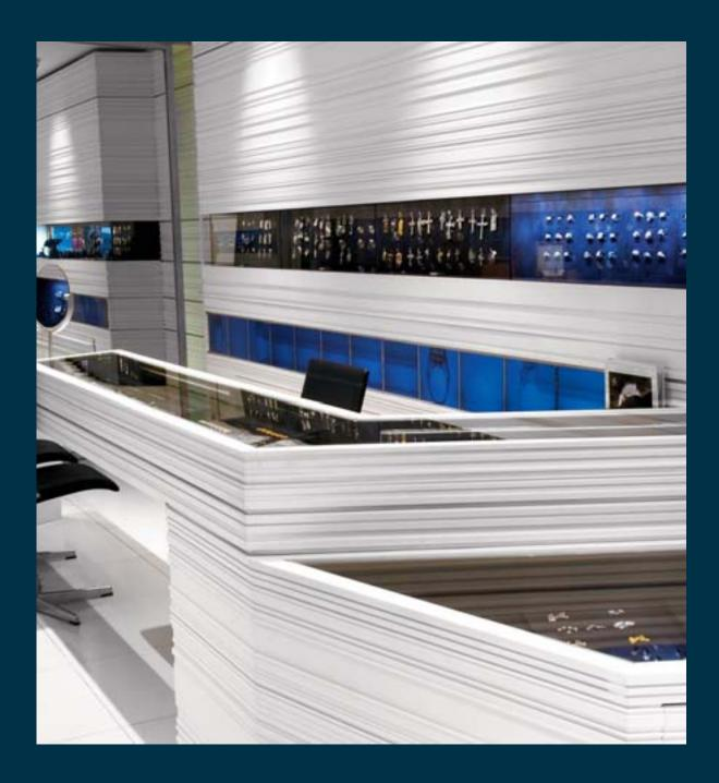
The seamless design flexibility of Corian® gives Jacob & Co. a contemporary linear look from the exterior cladding to the interior walls and displays. By digitally carving the Corian®, using a Computer Numeric Control (CNC) routing technique, the Arnell Group created a horizontally layered look mimicking the natural rock strata found in diamond mines.
